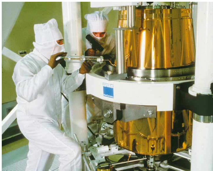
The high-precision X-ray mirror is inserted into the ROSAT satellite with extreme accuracy. The mirror, manufactured by the company Zeiss, set new records in terms of surface smoothness and shape precision.
